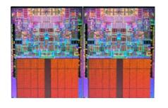
Intel Quad Core Duo Four identical x86 processor cores Separate L1 caches, shared L2 cache and main memory
