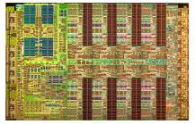
IBM Cell Broadband Engine One general-purpose PPE w/ 32K L1 caches and 512K L2 cache
