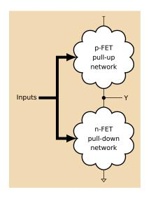
Pull-up and Pull-down networks must be complementary; exactly one should be connected for each input combination.
