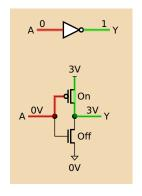
When the input is near ground ("0"), the p-FET is turned on, connecting the output to the power supply ("1"); the n-FET is turned off. p-FETs are only good at passing 1's
