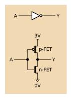
An inverter is built from two MOSFETs: An n-FET connected to ground A p-FET connected to the power supply
