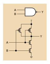
Two-input NAND gate: two n-FETs in series; two p-FETs in parallel
