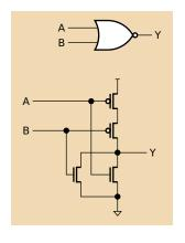
Two-input NOR gate: two n-FETs in parallel; two p-FETs in series. Not as fast as the NAND gate because n-FETs are faster than p-FETs
