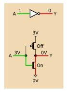
When the input is near the power supply voltage ("1"),
