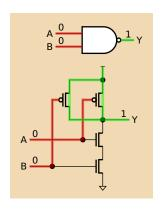
Both inputs 0: Both p-FETs turned on Output pulled high
