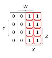
$$(W + \overline{W})X\overline{Y}\overline{Z} + (W + \overline{W})XY\overline{Z} + (W + \overline{W})XYZ + (W + \overline{W})X\overline{Y}Z$$
