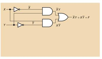
$$F = \overline{X}Y + X\overline{Y} = (X + Y)(\overline{X} + \overline{Y})$$
