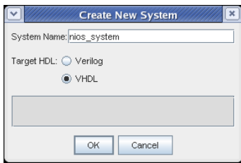
Figure 3: Naming a new system in SOPC Builder
