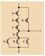
(b) Draw the schematic for a static CMOS gate that implements  $Y = \overline{(AB + C)D}$
