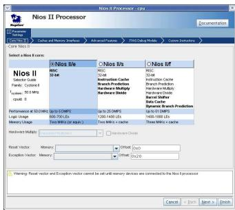
Figure 5: Adding an Nios II processor in SOPC Builder
