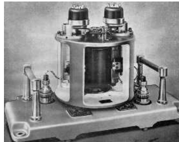
Magnetic drum memory. 1950s & 60s. Secondary storage.
