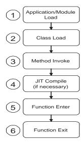
Figure 3: First method invocation in a Managed Application
