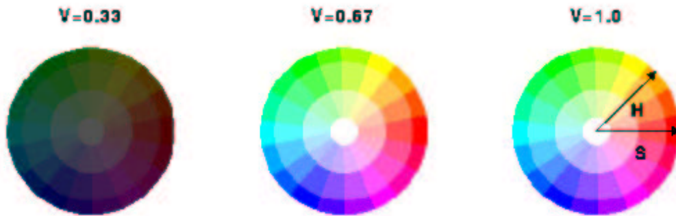
Figure 8.1: The quantized HSV color space, as shown here, allows for 18 hues, three saturations, and 3 values (plus four grays not shown).
