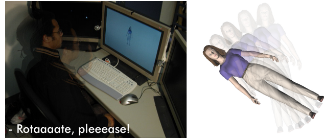
Figure 1. A desktop user manipulating a 3D model with speech commands, simple head gesture (tracked with audio) and speech rate. Rotation (shown at right) occurs after speech recognition.
