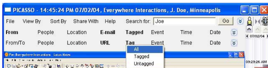
Figure 10 Searching for E-mails from Joe OR URLs shared by Joe. Notice the query being specified with the expanded Filter Panel.
