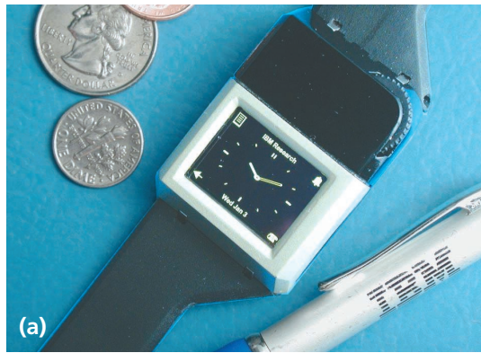
Figure 1. IBM wrist-watch computer with (a) OLED and (b) LCD display. The slightly larger LCD watch features auxiliary card housing under the wheel.
