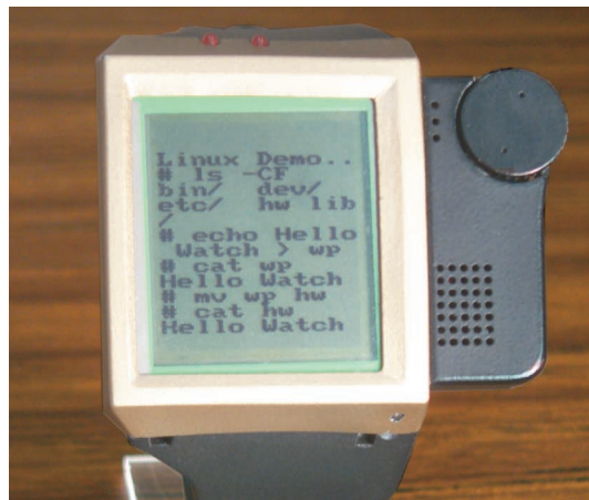
Figure 6. Linux shell loop demo. The demo program executed basic commands to show that Linux was running on the watch.
