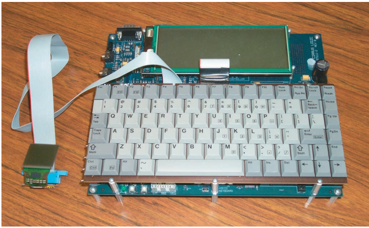
Figure 5. Cirrus Logic development board with liquid crystal display. The LCD was used first on the development board and then on the test bench before finally moving the code to the actual watch.
