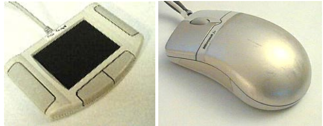
Fig. 1 Input devices for our desktop two-handed interaction techniques: a touchpad for the nonpreferred hand and the TouchMouse, a modified Microsoft IntelliMouse that can sense when the user is touching it.
