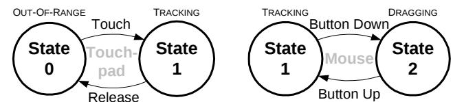
Fig. 4 State models for a touchpad (left) and a standard mouse (right).
