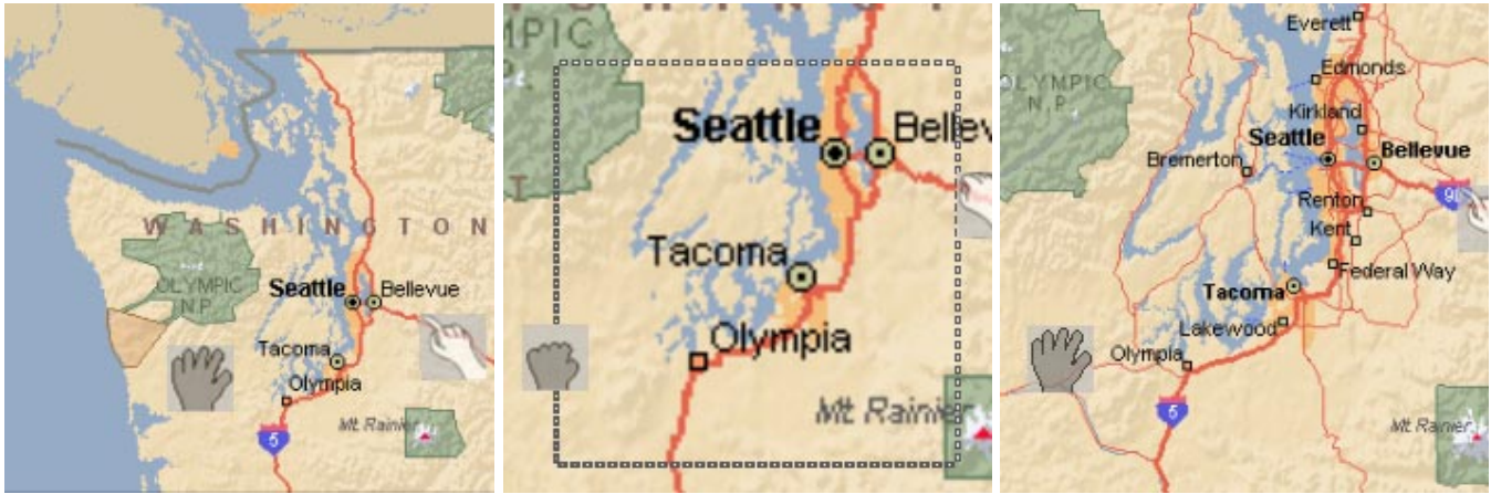
Fig. 5 Stretching the map with the TouchMouse and touchpad. The user first positions the cursors around an area of interest (left). Clicking and dragging the mouse and touchpad stretches the map; a dragging rectangle helps to show the area of the map that has been “grabbed” (middle). When the user releases the mouse button, the map updates, filling in additional detail (right). The new map fades in (as a 1 second animation) to reduce any visual discontinuities.
