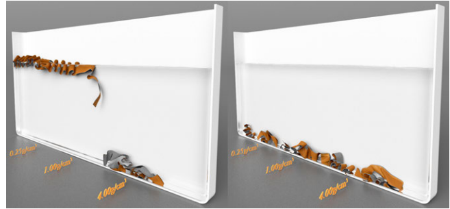
Fig. 4. Comparison with and without the liquid pressure gradient applied to solid. A simulation with the liquid pressure gradient applied to cloth yields correct buoyancy (left), where cloth lighter than water floats and cloth heavier than water sinks. Without the pressure gradient, all the cloth erroneously sinks (right).
