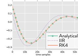
**Fig. 3: Comparison between Runge-Kutta and IIR filter:** Given a time-varying vibration equation, fourth-order Runge-Kutta (RK4) integrator (orange) offers higher accuracy against the IIR filter (purple), which was used in previous methods.
