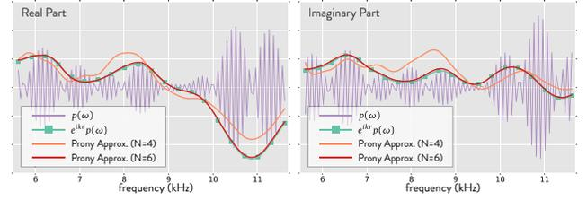
Fig. 6: **Frequency-Sweeping Transfers**: We choose one mode of the BUNNY model, evaluate  $p(\omega)$  using BEM at a fixed point as frequency sweeps and plot both real and imaginary parts.  $p(\omega)$  oscillates dramatically (purple); factoring out  $e^{-ikr}$  produces a much smoother curve (green); 4th-order Prony series gives a coarse interpolation curve (orange), while 6th-order series produces a curve (red) almost identical to the original function.
