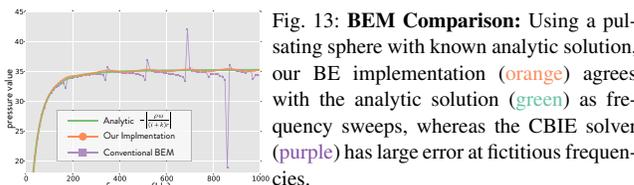
Fig. 13: **BEM Comparison:** Using a pulsating sphere with known analytic solution, our BE implementation (orange) agrees with the analytic solution (green) as frequency sweeps, whereas the CBIE solver (purple) has large error at fictitious frequencies.
