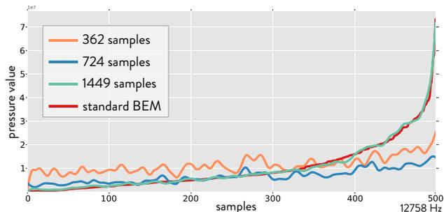
Fig. 12: **Convergence of Least-Squares Approximation:** Fixing the frequency value  $f = 12758 Hz$ , we estimate  $M_n^m$  using an increasing number of key positions. We use the estimated  $M_n^m$  to evaluate acoustic transfer values at 500 randomly selected locations (orange, blue, and green curves), and compare them against accurate transfer values solved using conventional BEM (red). As the number of key positions increases, we get higher fidelity for the estimated transfer values.
