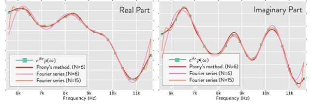
Fig. 16: **Prony Series vs Fourier Series:** We compare the approximation of frequency-dependent pressure curves using Prony series and Fourier series. The ground-truth pressure curves are the same as the ones in Figure 6. We plot the Prony approximation using 6 terms, and Fourier approximation using 6 and 15 Fourier basis functions respectively.
