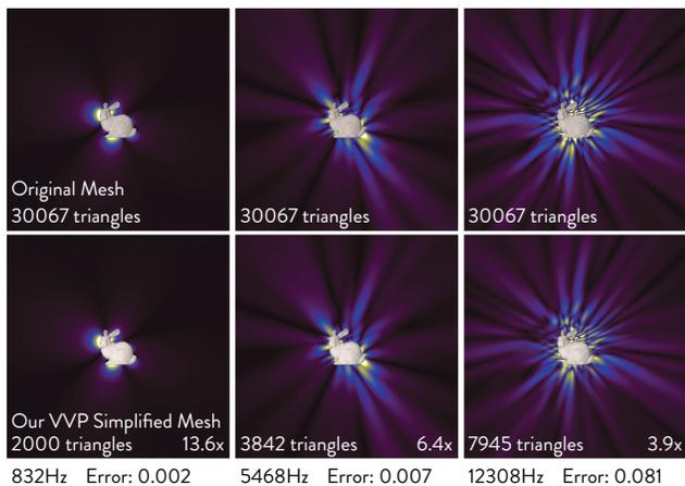
Fig. 10: **Transfer Values with Frequency-Adaptive Remeshing:** We compare transfer values computed using the original high-resolution mesh (top) with the values using simplified meshes (bottom) for three modes with low, medium and high frequency values. Even for high-frequency modes which require a relatively high-resolution mesh, our method achieves nearly  $4\times$  speedup, while retaining a low  $L_2$  error ( $< 8.2\%$ ).
