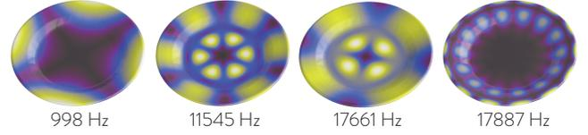
Fig. 8: **Smooth Modal Shapes:** Color encodes the modal displacement amplitude of the PLATE model; modal frequencies are listed below each subfigure. Even for high frequency modes, their modal displacement varies smoothly on the surface, making it possible to perform mesh simplification.
