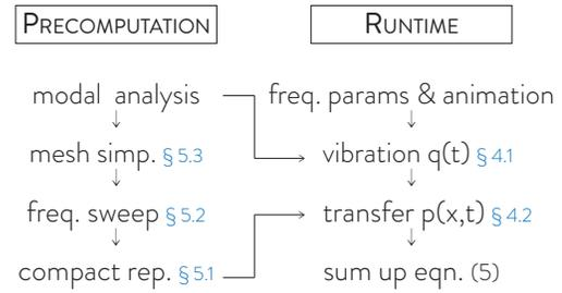
Fig. 2: **Overview:** given an input mesh, we efficiently perform the precomputation (left). At runtime, given a rigid animation, we can then quickly synthesize resulting rigid-body sounds with user-specified frequency parameters (right).
