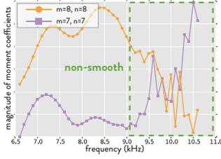
Fig. 4: **Non-smoothness of  $M_n^m$** : The high-order  $M_n^m$  becomes non-smooth and fluctuates strongly at high frequencies, making direct interpolation difficult. We note that these orders (i.e.,  $N=7,8$ ) are necessary in the expansion for sufficient accuracy.
