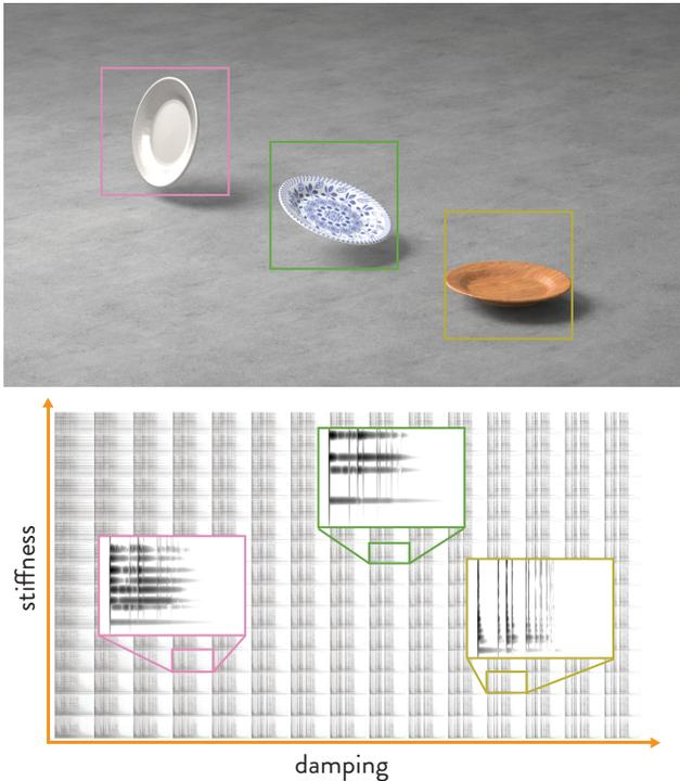
Fig. 1: **Parameter Exploration using our method:** With our precomputed information, we are able to explore the space of modal sound parameters at runtime, achieving numerous sound effects (bottom) synchronized with a physics-based animation. The three spectrograms highlighted in the colored boxes correspond to (left to right) metal, porcelain, and wood materials shown on the top. We refer to this link for all 225 sounds shown here. <http://www.cs.columbia.edu/cg/interactivetransfer/>
