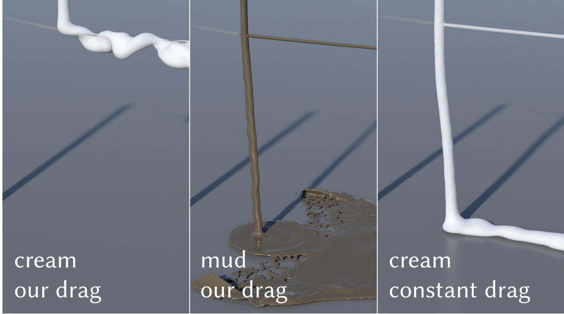
Figure 13.9: Comparison of different drag coefficients. Streams of shaving cream and mud are poured onto seven hanging strands. Left and middle: Our drag model yields very different interaction behavior depending on the liquid type; Right: A constant drag coefficient, on the other hand, produces a drag effect for the shaving cream similar to that of mud, since the yield stress and viscosity are not considered.
