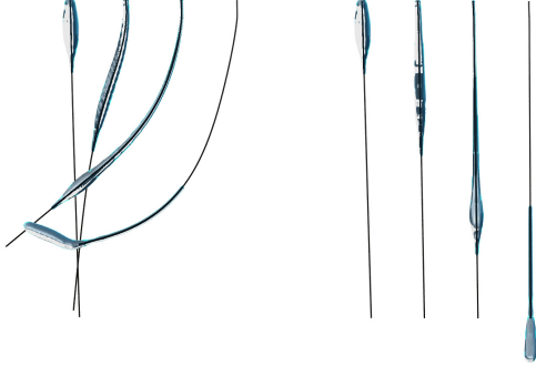
Figure 8.7: A droplet sliding down a single vertical hair as it moves under uniform horizontal velocity. Under (only) downward gravitational acceleration, the hair should remain vertical, in the absence of external horizontal forces. We compare naïve local momentum rescaling (left) versus our momentum update transport (right) .
