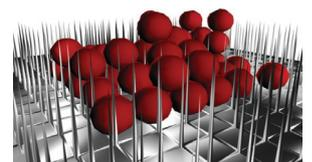
**Figure 11. Experiments with a bed of nails highlight the method’s ability to deal with sharp boundaries, isolated points of contact, sliver triangles, and localized points of high pressure between two nearly incident surfaces.**
