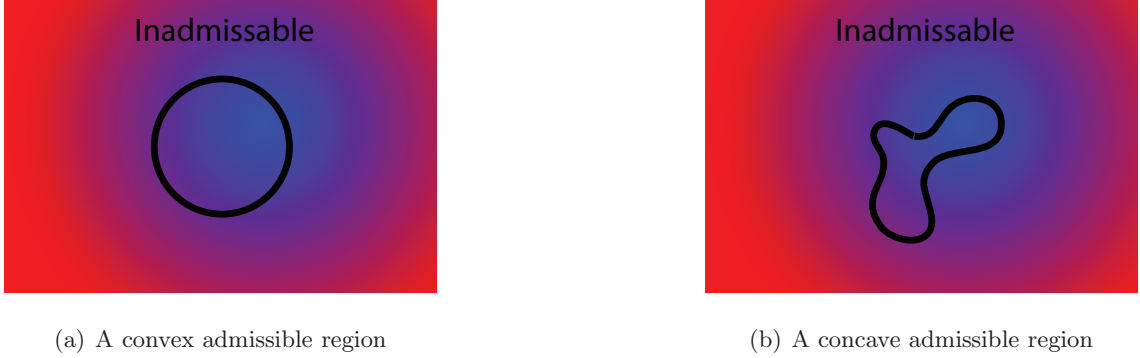
Figure 3.4: The importance of convexity in constraint satisfaction
