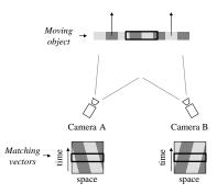
Figure 3: Distortions in temporal stereo caused by a moving object. The matching vector is drawn in 2D with one spatial dimension and one time dimension. Rows in the matching vectors represent moments in time. Although the highlighted time instant is in direct correspondence, the temporal neighborhood has been subjected to distortion.
