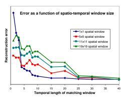
Figure 10: Error as a function of spatio-temporal window size for the wood-block scene illuminated with a flashlight.
