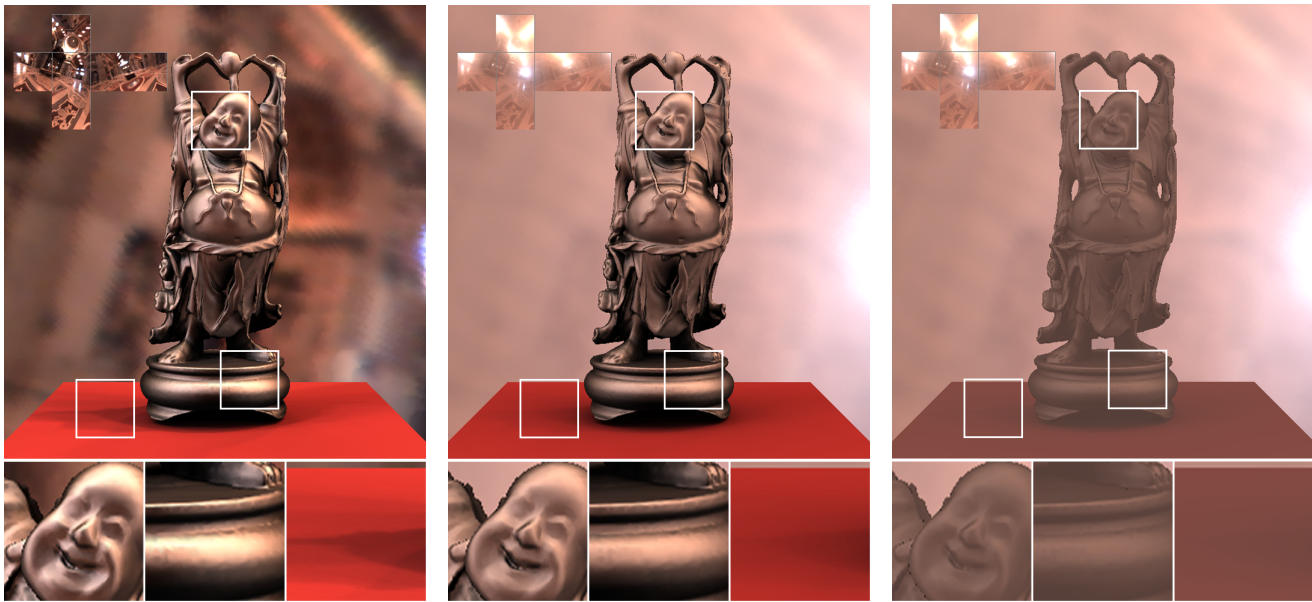
Figure 16: [Left] A scene rendered using precomputed radiance transport, to capture the complex shadows and specular surface BRDFs. [Middle] The same scene rendered as though it was immersed in a scattering medium, with the observer close to the object. Notice the blurring and fogging of the environment in the background. In the insets, we see a number of shading changes, such as the brightening of dark regions in the face because of the scattering of light, the attenuation due to dimming and diffusing of specular highlights on the base, and the softening of shadows on the plane. [Right] The same scene including effects of airlight between viewer and object (as if the viewer were far away, seeing the Buddha through fog). Note the loss in contrast and saturation.
