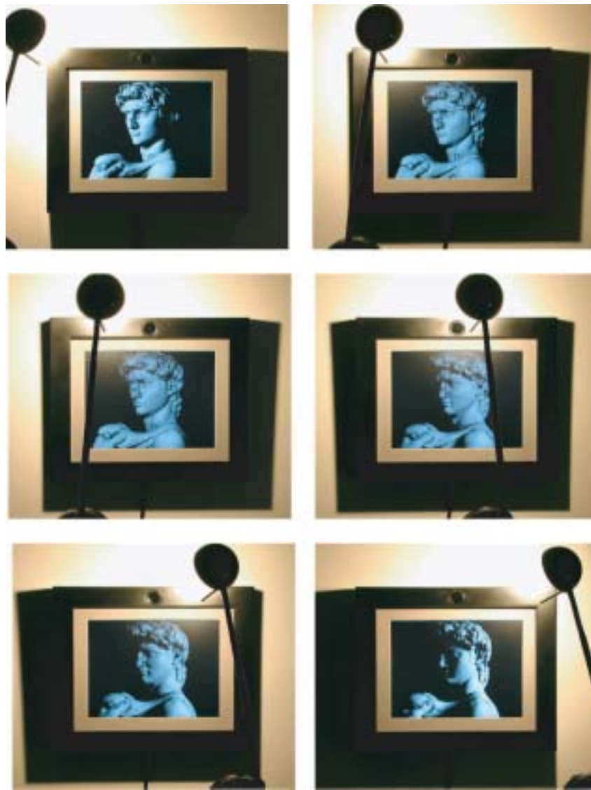
Fig. 8. LSD outputs for the David model corresponding to different illumination conditions. The complex shadows in the hair, eyes and neck regions are reproduced with the desired sharpness.
