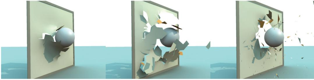
Figure 11: We simulate the puncture of an elastic sheet by a fast projectile. By varying the fracture threshold,  $\lambda_f$ , we obtain different behaviors. From left to right,  $\lambda_f = 0.02, 0.001, 0.0001$ .
