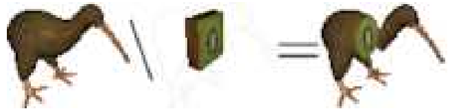
Figure 11: We retain the relationship between the output triangles and the inputs. Because of our exactness, attributes like texture coordinates are losslessly maintained.
