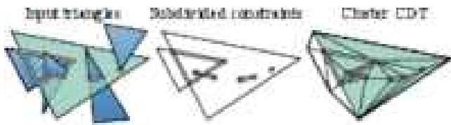
Figure 9: Blue triangles intersect the green at a point, segments and a polygon (left, 3D). Subdivided constraints reduce to coplanar points and segments (middle, 2D). The original green triangle is replaced with replications of the green triangles of a constrained Delaunay triangulation (CDT) of the coplanar cluster (right, 2D).
