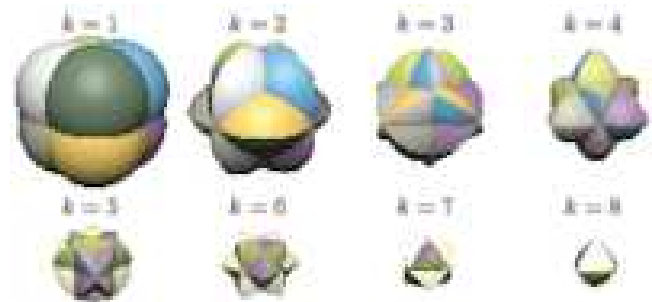
Figure 31: Our method supports n -ary operations. For example, extracting all regions inside at least k of the input spheres centered at each corner of the unit cube.
