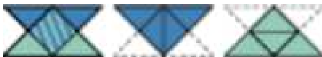
Figure 10: Two overlapping, co-planar right triangles (left) admit multiple constrained Delaunay triangulations (CDTs). Independent triangulation could lead to inconsistency (middle and right).
