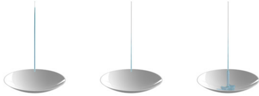
Fig. 12. Reduced-liquid flow and dripping on a single strand. Left: No reduced-liquid flow. Center: Reduced-liquid flow without dripping; the liquid flows towards the tip and disappears. Right: Reduced-liquid flow with dripping enabled.
