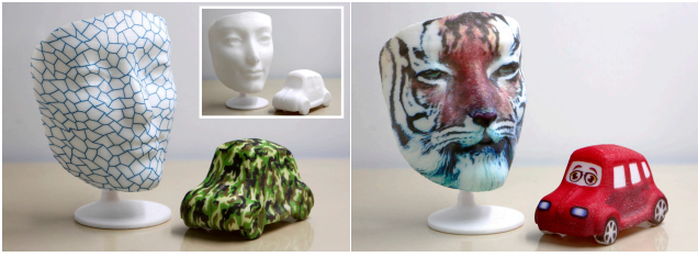
Figure 2: Traditional method vs our method. (left) Traditional hydrographic printing is mainly used for coloring 3D shapes (inset) with repeated color patterns, because it lacks a method to (i) map a surface texture to a printable 2D image and (ii) precisely register the color texture on surface. (right) Our method solves these problems, so user-specified color textures can be hydrographically printed.
