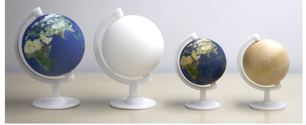
Figure 15: Globes. We make globes by transferring an earth texture to spheres. From left to right, the second and fourth models are the original spheres made by plastic (3D printed) and wood, respectively. The first and third are the ones with hydrographically printed textures on both materials.
