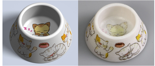
Figure 17: Failure case. When we color the bottom surface of a cat bowl, the PVA film has been extremely stretched (or even broken) before adhering to the surface, resulting in deteriorated printing quality: (left) the desired surface texture and (right) our hydrographic printing result.
