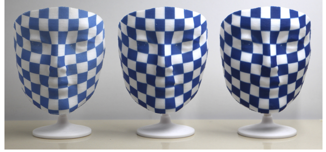
Figure 11: Repeatability. We color a single facial model multiple times, each with the same chessboard pattern and hydrographic printing setup. From left to right, the surfaces are hydrographically printed once, twice and three times, respectively.
