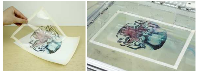
Figure 3: PVA film with a printed color pattern. (left) The PVA film is attached on an A4 paper, so it can be fed into a conventional inkjet printer to print prescribed color patterns. (right) the film is put on water and ready for transferring colors to an object surface.
