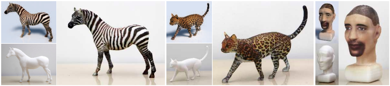
Figure 16: Multi-immersion printing. For such complex models as zebra (left), cat (middle) and the head (right), we perform multi-immersion printing as introduced in §6.
