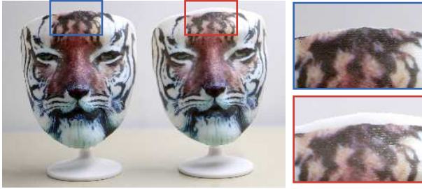
Figure 7: Influence of film thickness. We compare the texture alignment with and without nonuniform film thickness considered in the simulation. (left) We use the two-step simulation introduced in §4.3 to compute the printed image for hydrographic printing. (right) We assume a constant film thickness in the simulation for computing the printed image pattern.
