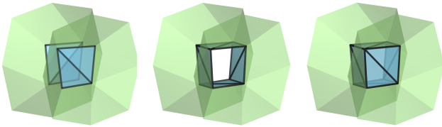
Fig. 16. Zipper-based merging: Left: Two nearby edges are identified, with incident triangles shown in blue. Deleting these triangles produces a quad-shaped hole in each surface. Middle: If the materials on their interiors are the same, the holes are zippered together to produce a connecting tube. Right: If the materials differ, one of the triangle-pairs is left in place but with its labels modified, to maintain separation of the materials.
