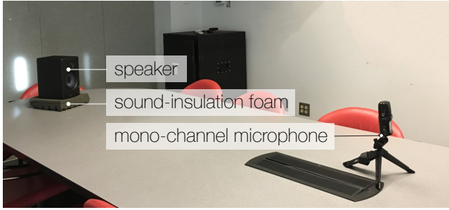
Fig. 4. IR measurement. We measure the IR using a conventional speaker and a mono-channel microphone. The speaker plays a sine sweep noise, which is then recorded by a microphone. In practice, we put the speaker on soft foam to absorb any mechanical vibrations it produces, which can be propagated to the microphone through the table.
