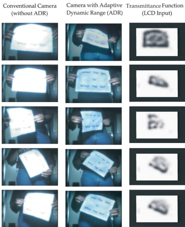
Figure 7: A scene with a bright sheet of paper. While the paper is saturated in the case of a conventional camera (despite the use of AGC), the crumpling of the paper and the text on it are clearly visible in the case of the ADR camera. Note the spatio-temporal adaptation of the attenuation function shown in the right column.
