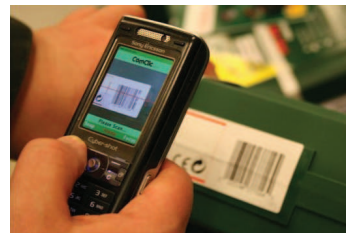
Figure 1: Some cellphones can read a bar-code and search for product information online. The user can then choose to purchase the item (from Amazon Mobile, 2004). The optical tag projection and detection method described in this paper enables the same functionality, but without physically attaching hardware tags on objects.
