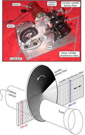
**Figure 1.** A system for demonstrating the algorithms of uncontrolled modulation imaging. It uses a monochrome image detector. Adjacent to the detector (before the lens), there are two spatially varying filters: one with varying transmittance, the other with a varying spectral response.
