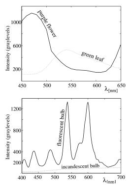
**Figure 9.** Experimental results. Spectral plots extracted from video streams, samples of which are shown in Fig. 5. The correspondence between intensities and wavelengths was achieved using computational synchronization. The HDR intensity values in the plots are obtained thanks to the multiple transmittance (exposure) settings used.
