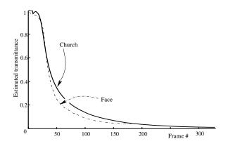
**Figure 3.** The estimated transmittance as a function of time (frame index), for two video streams. The transmittance was calculated based on the raw images, bypassing the need for imaging synchronization.
