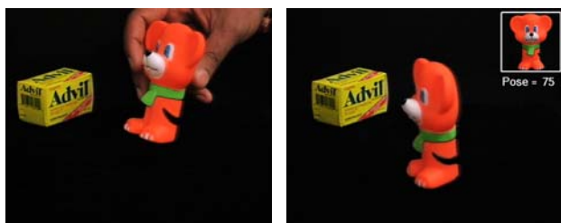
Figure 1: The Columbia Object Image Library (COIL-100) contains 7,200 images of 100 objects. (a) The objects have a wide variety of complex geometric and reflectance characteristics. A real-time 100 object recognition system was constructed using COIL-100. (b) A toy cat from the database is shown to the system for recognition. (c) The system recognizes the object in less than one second. The recognized object and it's pose are displayed in the upper right hand corner.
