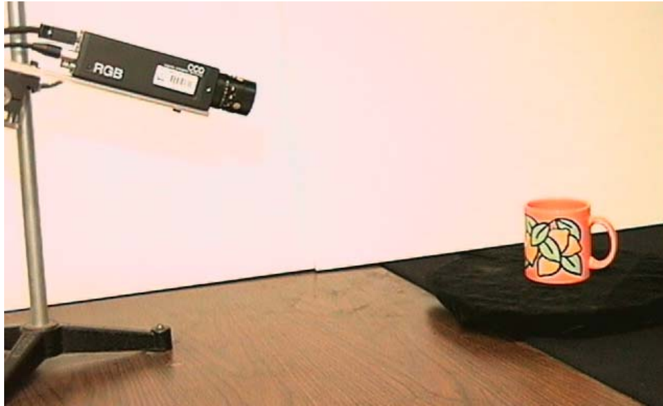
Figure 2: The objects were placed at the center of a motorized turntable. The turntable was rotated through 360 degrees. An image was acquired with a fixed color camera at every 5 degrees of rotation.
