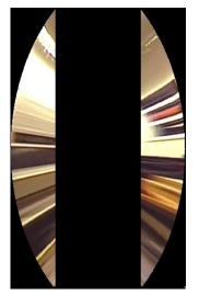
Figure 12: Two 90 degree sections of a cone are projected on to the larger dimension of the rectangular image. This results in a panoramic slice camera with a two-fold increase in slice resolution.
