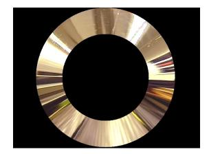
Figure 9: Example of an image produced by the slice camera shown in Figure 8. As expected, scene features are projected to radial strips in the image.
