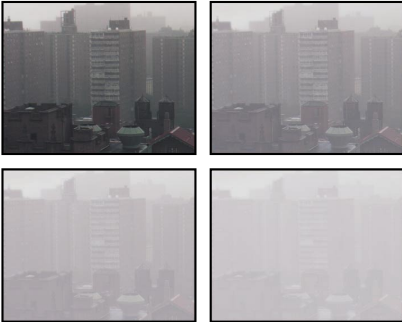
Fig. 13. Generation of novel images with increasing fog densities (or scattering coefficients). The relative scattering coefficients used in this case are \beta , 2\beta , 3\beta and 4\beta respectively.
