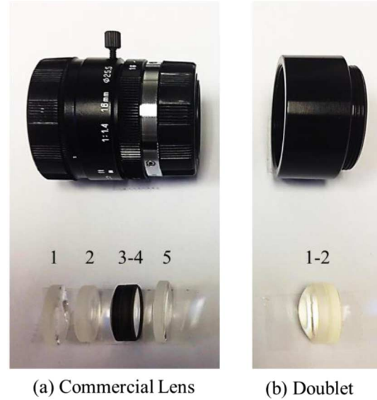
Fig. 10. Lens Simplification. (a) A commercial lens (with five elements), and (b) a simplified lens (with two elements) that produces similar image quality when used with a focal stack or focal sweep.
