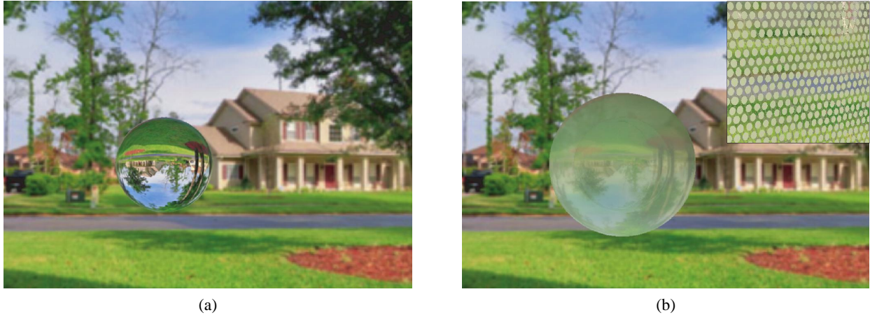
Figure 4: Rendering of a spherical image capture and display device: (a) A ball lens ( \mu = 1.5 ) is placed at the center of a spherical environment map. (b) Consider a detector shell built around the ball lens in which the sensors are replaced by a thin translucent material that diffuses light in all directions. The lens forms an image of the environment on the inner surface of the translucent shell. Owing to the diffusing nature of the shell, the image is also visible from outside the shell. The figure shows a rendering of such a system that can simultaneously capture and display spherical environments. The inset shows a small portion of the spherical diffuser shell showing the individual translucent pixels.
