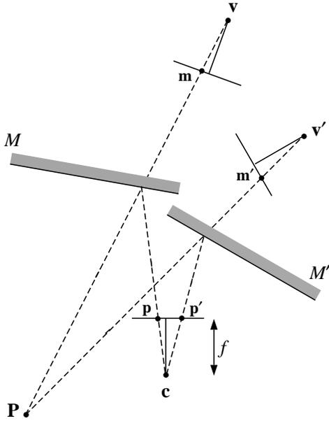
Figure 1: Stereo image formation with a single camera and two planar mirrors. A scene point  $P$  reflected off mirrors  $M$  and  $M'$  is imaged as if seen from two different viewpoints  $\mathbf{v}$  and  $\mathbf{v}'$ .
