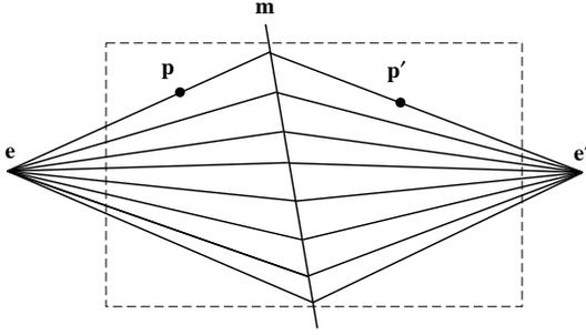
Figure 2: The epipolar geometry of planar motion. When motion is constrained to lie in a plane, all corresponding epipolar lines must intersect at  $\mathbf{m}$  the image of the axis of rotation. Therefore, the two epipoles  $\mathbf{e}$  and  $\mathbf{e}'$  and the line  $\mathbf{m}$  completely determine the epipolar geometry.
