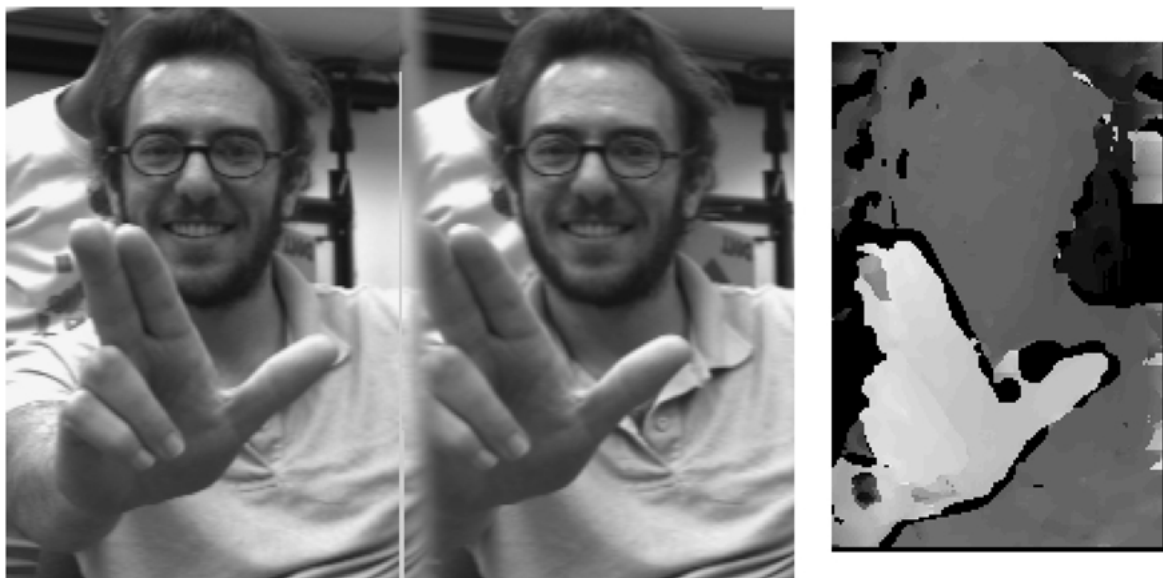
Figure 13. Stereo image and depth map. On the left is an image taken by a catadioptric stereo system and on the right is the depth map computed with the SAD measure and a 7 \times 7 window.
