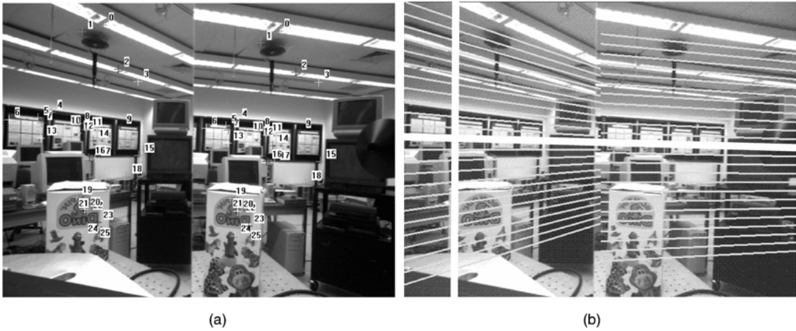
Figure 7. (a) A set of image correspondences used to compute the epipolar geometry. (b) The recovered epipolar geometry. The vertical thick line is \mathbf{m} the estimated image of the screw axis, where the corresponding epipolar lines meet. The horizontal thick line is the line connecting the two epipoles, the horizon line of the planar motion. The intersection of the two lines is \mathbf{m}' and is used to estimate the focal length.
