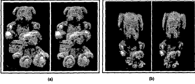
Figure 1: Not all rectified images are the same. (a) On the left is a pair of rectified stereo images. (b) The images on the right are also rectified, however, due to a poor choice of the rectifying transformation a large amount of under-sampling and over-sampling exists which makes stereo matching difficult.
