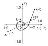
Fig. 3. Mapping the impulse responses to an optimal linear space. The transformed discrete points form a trajectory in the n-dimensional linear space. This figure shows the three dominant dimensions of the linear space. If the dynamical system is stable, the trajectory finally converges to the origin.
