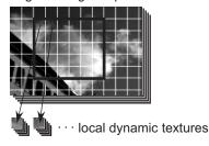
Fig. 1. Local dynamic textures are defined as the dynamical properties of small spatial regions of an image sequence. In this figure, the image is partitioned into several blocks, each block with its own dynamical model.
