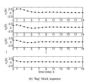
Fig. 8. Impulse responses computed for (a) a 'snow' block sequence (the 15th block) and (b) a 'flag' block sequence (the 15th block). In this case, n=10.
