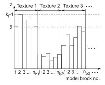
Fig. 5. An example histogram of the number of closest points between trajectories. Since two different types of dynamic textures can have many points close to each other, the similarity between two trajectories is evaluated only if the number of closest points exceeds the threshold  $\bar{z}$ .
