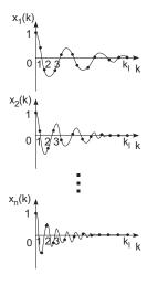
Fig. 2. Impulse responses of state variables of the estimated dynamical model. For an n-dimensional state space, n impulse response sequences are obtained. In the case of discrete time sequences each sequence consists of  $k_l + 1$  ( $k_l$  is the terminal time index) discrete points.
