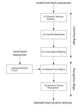
Fig. 4. Dynamic texture recognition scheme. The proposed recognition system is divided into two stages; a learning stage and a recognition stage. In the first stage, the point sets (trajectories) in the optimal linear space corresponding to each block (local texture) of the image sequence are computed. In the next stage, the dynamic texture recognition is applied to each block of a novel image sequence.
