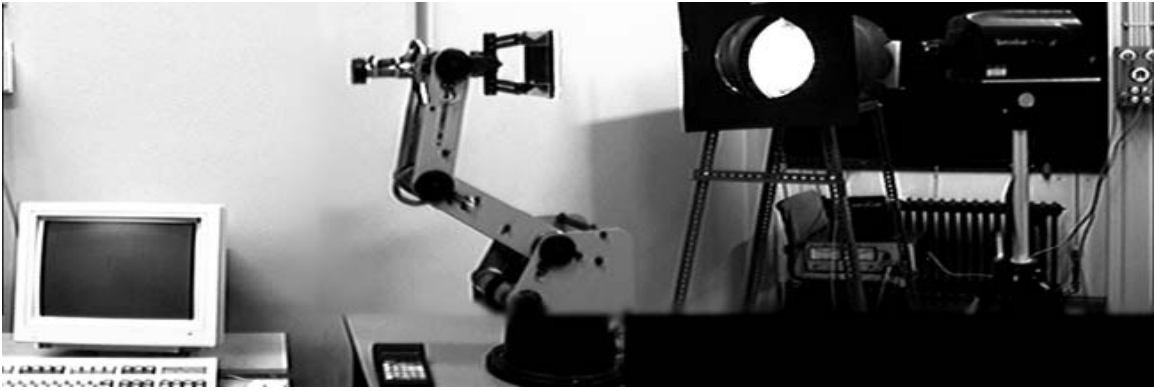
Figure 3: Measurement setup. The equipment consists of a personal computer with a 24-bit R/G/B frame grabber, a robot arm to orient the texture samples, a halogen bulb with a Fresnel lens which produces a parallel beam, a spectrometer and a 3-CCD color video camera (not shown).
