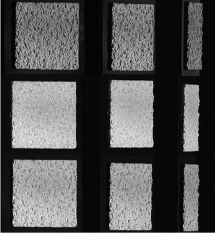
Figure 7. Images of rough plaster (sample 11 in the texture database) taken under 9 different illumination and viewing directions. From left to right the columns correspond to \theta_v = 33.75^\circ, 56.25^\circ and 78.75^\circ . From top to bottom the illumination polar angle is \theta_s = 11.25^\circ, 33.75^\circ and -11.35^\circ .
