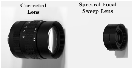
Figure 2. A comparison showing the relative sizes and complexities of a Cosmimar 75mm F/1.4 lens (left) and our F/4 SFS doublet lens (right). Our lens is significantly lighter and more compact. The corrected lens is stopped down to F/4 in all experiments.
