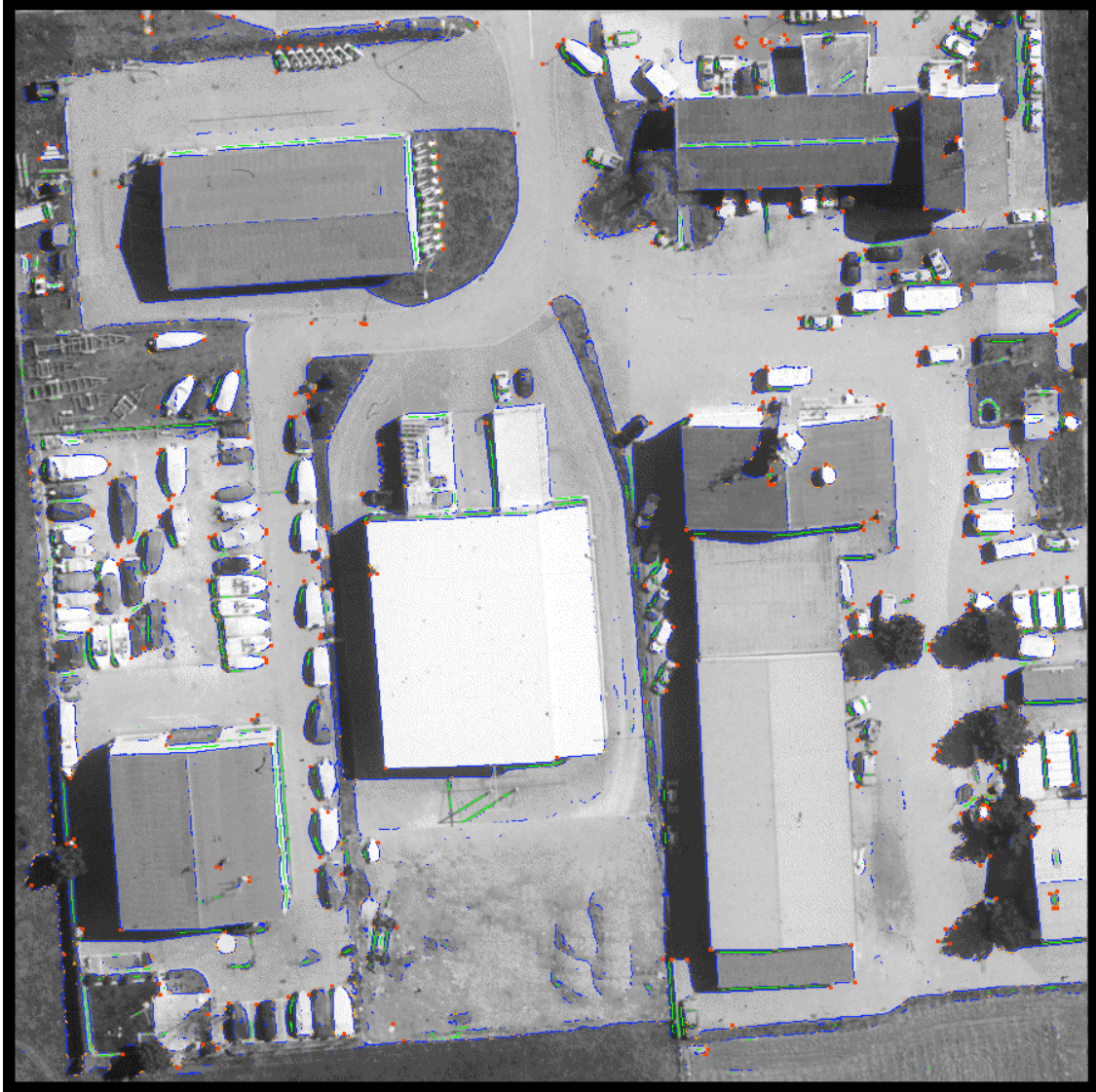
Figure 4.15: The results of applying the step edge, corner, line, and circular disc detectors to the 900 \times 900 pixel image “INRIA Bulding.” Step edges are overlaid in blue, corners in red, lines in green, and circular discs in yellow.
