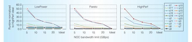
Figure 5. Most TPC-H queries are not sensitive to the Q100 intraconnection throughput, except for Q10, Q16, and Q11. These queries process large volumes of records throughout the query with little local selection conditions to funnel down the intermediate results. When network-on-chip (NoC) bandwidth is constrained, these queries could execute 50 times slower.
