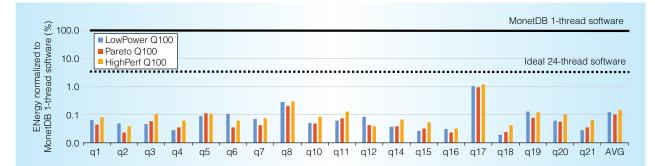
Figure 12. TPC-H query energy consumption normalized to MonetDB single-thread running on cores consuming non-idle power shows 691 to 983 times energy efficiency on average across all queries.
