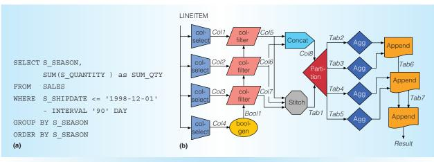
Figure 1. An example query for producing a summary sales quantity report. (a) A SQL query and (b) the corresponding Q100 query plan, where nodes represent relational operators, and the edges between them are data dependencies.
