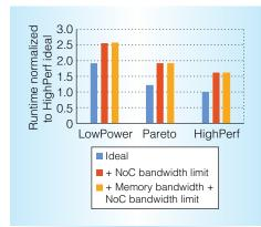
Figure 10. From the bandwidth heat maps plotted earlier, we see that Q100 was demanding a lot more NoC bandwidth than provisioned. Here, we plotted runtime with respect to no bandwidth-limit penalties, and we see a large slowdown at 30 to 60 percent, a caution for future implementations to design sufficient bandwidth for intra-tile connections.
