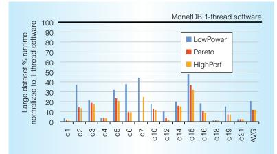
Figure 13. With a dataset that is 100 times the size of our previous input tables, TPC-H still shows a 10 times performance improvement relative to software on average.
