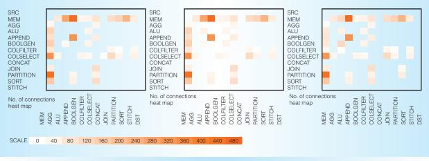
Figure 4. A heat map of tile-to-tile connection counts: (a) LowPower, (b) Pareto, and (c) HighPerf designs. Most intra-tile connections exist mostly when communicating to and from memory.
