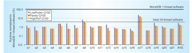
Figure 11. TPC-H query runtime normalized to MonetDB single-threaded software shows a performance improvement of 37 to 70 times on average across all queries.
