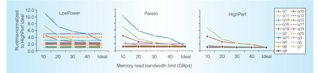
Figure 8. Similar to NoC bandwidth, most queries are not sensitive to memory read bandwidth. However, in the HighPerf design, more resources allow for a more efficient scheduling of temporal instructions, reducing high-volume communications to and from memory.
