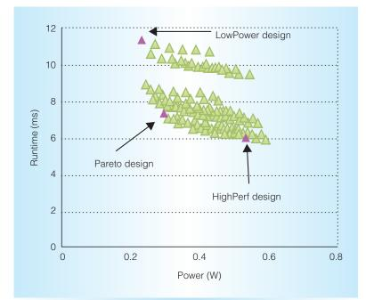
Figure 3. Out of 150 configurations, we selected three designs for further evaluation: LowPower for an energy-conscious configuration, HighPerf for a performance-conscious configuration, and Pareto for a design that maximizes performance per watt.
