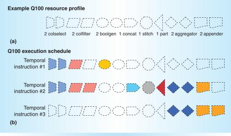
Figure 2. Given a Q100 instance with finite resources, as shown in (a), the query plan is broken into a sequence of temporal instructions by a scheduling algorithm that attempts to maximize resource usage and minimize data spillage between instructions.<sup>14</sup> In (b), the query plan from Figure 1 requires three steps to complete.
