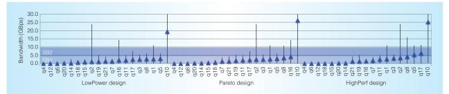
Figure 7. Write bandwidth demands are quite a bit lower than read bandwidth demands for most queries. We sized all three designs with two stream buffers, providing 10 Gbytes per second (GBps) write bandwidth to memory.
