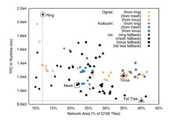
Figure 5: Design space exploration of semi-specialized NoC topologies. We compare our algorithm with Ogras et al. [19], Koibuchi et al. [15], and four generic topologies. We find that our approach to network specialization is the most effective, producing designs that approach the performance of a fat tree and have a smaller resource-cost than a simple double ring, which are indicated by the dashed lines in the plot.
