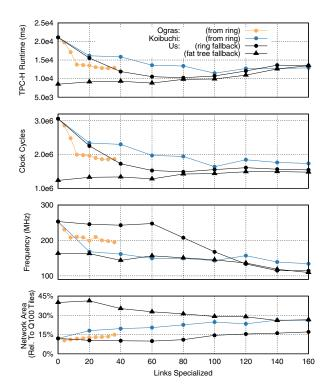
Figure 6: The best NoC configuration we found came from specializing 60 edges and employing a double ring fallback. This network is superior to those from other methods because our NoCs are more resource conscious.
