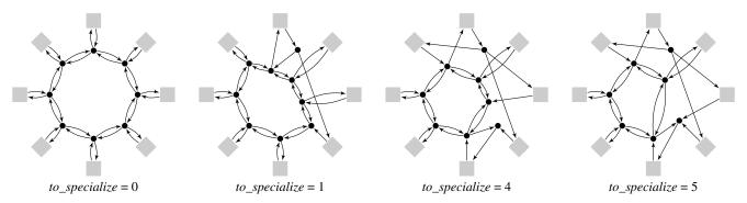
Figure 3: Networks produced by our algorithm employing a ring fallback for a certain system with 8 ports. More specialization steps produces a more customized network and a smaller ring.
