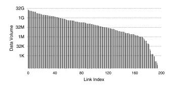
Figure 1: Motivation for limited specialization: the volume of link traffic falls off exponentially from the busiest links, suggesting only a handful of specialized links are necessary. (TPC-H on the Q100)
