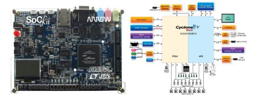
**Fig. 3.** The Terasic SoCKit Board [4] brought dual hard ARM9 cores via a Cyclone V FPGA, enabling the use of Linux software and its device drivers. The main failing of these boards has been the fragile micro-USB connectors.
