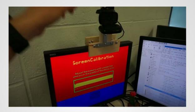
In order to make the function works, we have to make sure the camera can capture the area for touch detection. Thus, we provide user a convenient way to calibrate the screen position.
