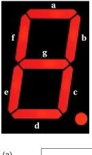
Figure 12: A seven-segment LED display. E.g., hex0(0) is a; hex0(6) is g
