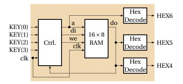
Figure 11: The block diagram of lab 1
