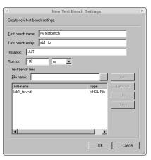
Figure 14: Telling Quartus about a new test bench
