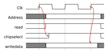
Bus cycle starts on rising clock edge. Peripheral latches data two cycles later. For slower peripherals.
